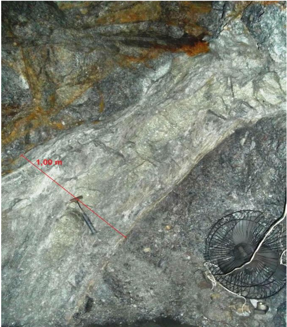
Figure 6. SE Face of -54 m level showing massive pyrite band.
