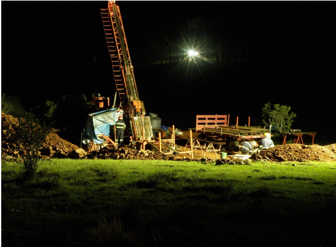
Figure 2: One of 4 Diamond Drilling rigs currently employed at CDS's Uruguayan operations.
